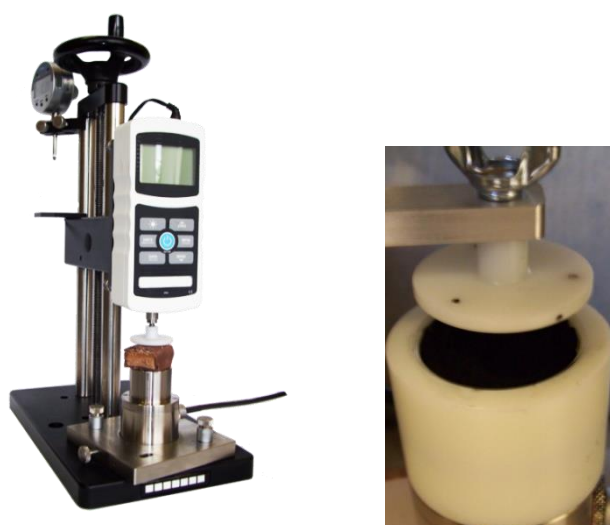
Figure 2. L: The C-Therm TCi's Compression Test Accessory. R: Toner being tested for thermal conductivity using the Compression Test Accessory with the extension applicator inside a thermal chamber.
