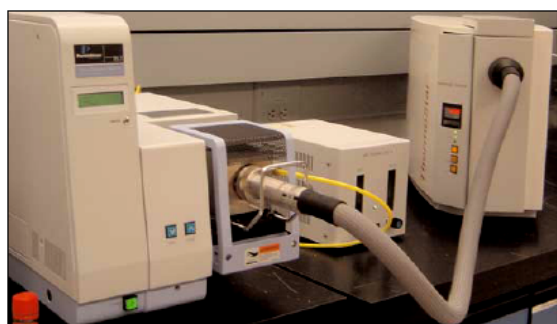
Figure 1. PerkinElmer Diamond TG/DTA (left) connected to a Pfeiffer ThermoStar MS (right). Cooling/Gas Switching Accessory (center) is also shown.
